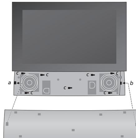
**Attaching the speaker cover:** Hold up the speaker cover slightly to the right of the 'brackets' a and b. Now slide the cover to the left to let the 'attach-points' engage with the corresponding 'brackets' (a, b and c) on the television.
