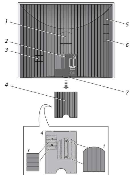
*The covers shown (1 and 3) can be kept inside the cover of the main socket panel.*
