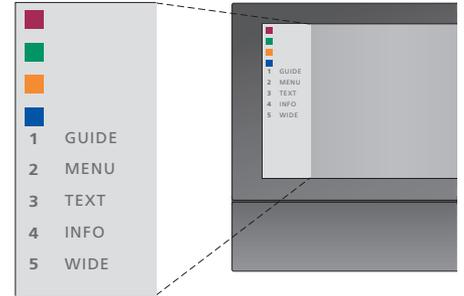
*Example of a Peripheral Unit Controller menu – The Beo4 buttons are shown to the left on the menu, and the functions they control are shown to the right. The menu may also list buttons on the remote control included with your connected equipment.*
