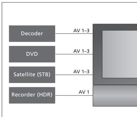
This diagram shows examples of additional video equipment that can be connected to the television at one time. If you have a Bang & Olufsen recorder, it must be connected to the AV1 socket.
