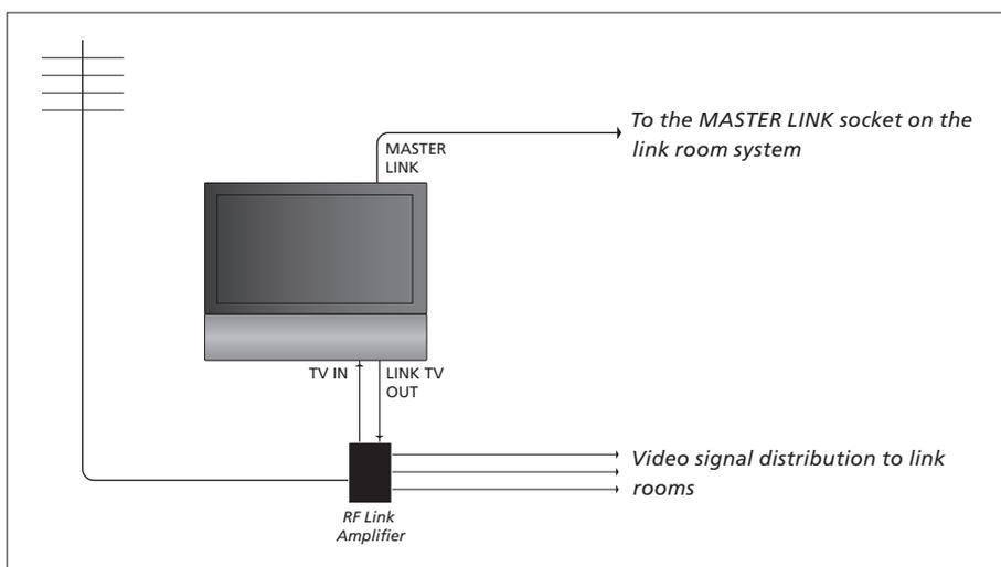
**The main room system must be connected to the link room system with a Master Link cable.**
